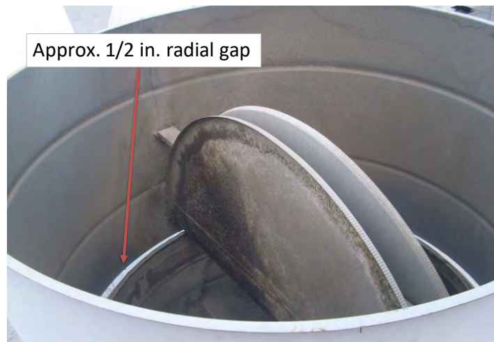
Figure 2: Illustration of Radial Gap between Fan Barrel Diameter and Butterfly Damper Barrel Diameter
